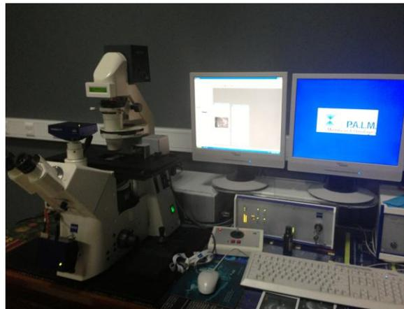
*P.A.L.M. laser microdissecting microscope*
