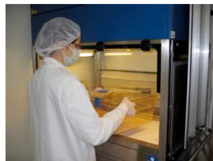
Laminar flow chamber
