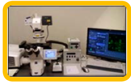
Confocal Microscope Zeiss LSM 710 which includes 3 R7FL spectral channels, 5 laser lines: 458, 488, 514, 561 and 633
