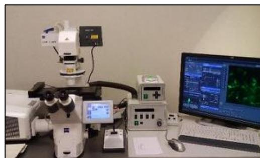
Confocal Microscope Zeiss LSM 710 which includes 3 R7FL spectral channels, 5 laser lines: 458, 488, 514, 561 and 633
