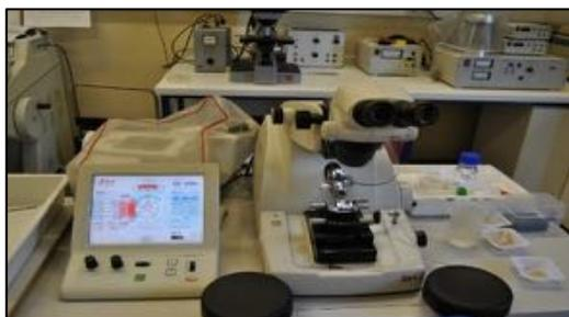
Leica ultramicrotome with a cryo unit (EM UC6 and EM UC6A)
